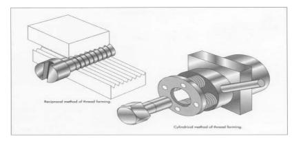
Threads can be cut into the blank by several methods. In the reciprocal method, the screw blank is rolled between two dies. In the cylindrical method, it is turned in the center of several rollers.
